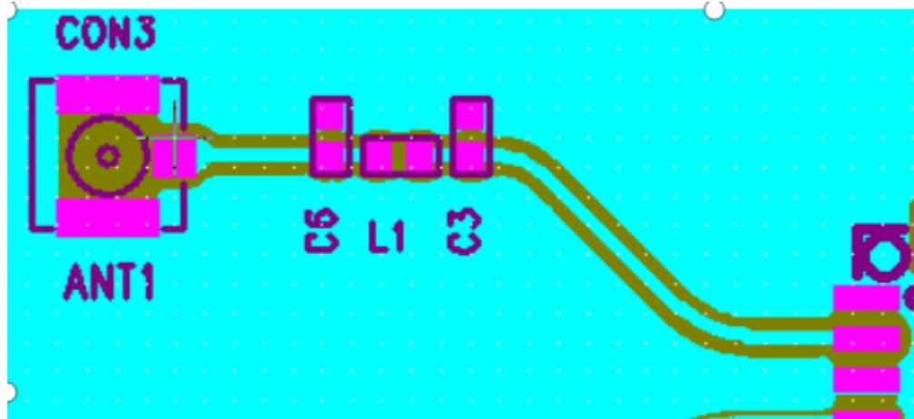
The module needs to be attached to the PCB board and connected to the external antenna through the solder joint of the circuit on the PCB. The gain of the external antenna is 2dB( Max. ), the internal structure is copper tube structure or FPC. A resistance of 0R is added between the module and the antenna at L1 to ensure that the impedance of the connection between the module and the antenna reaches 50R. The ANT1 position on the PCB is where the external antenna is connected.
